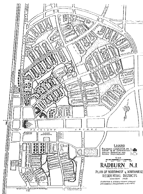
Figure 6.10. Plan of Radburn, New Jersey, showing houses facing inward onto parks that connect throughout the development. (Source: Clarence Stein, Toward New Towns for America , 1951)
