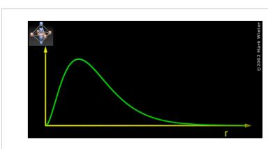
Schematic plot of the 1s radial distribution function  $4\pi r^2\psi_{1s}^{\phantom{1}2}$
