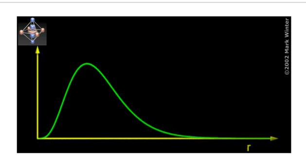
Schematic plot of the 2p radial distribution function  $r^2R_{2p}^2$  ( $R_{2p}$  = radial wave function).
