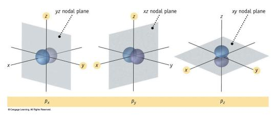
The three degenerate p-orbitals spread out on the x, y & z axis, 90° apart in space.
