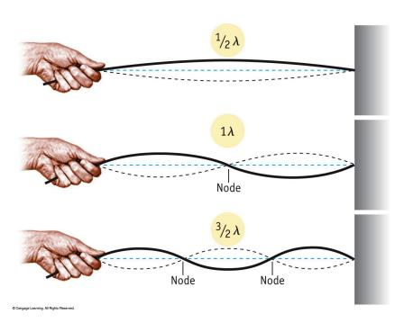
Wave motion: wave length and nodes "Quantization" in a standing wave
