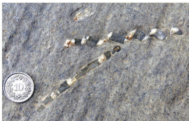
Figure 3.1 Two elongated belemnites in Jurassic limestone in the Swiss Alps. The different ways that the two belemnites have been stretched give us some two-dimensional information about the strain field: the upper belemnite has experienced sinistral shear strain while the lower one has not and must be close to the maximum stretching direction.
