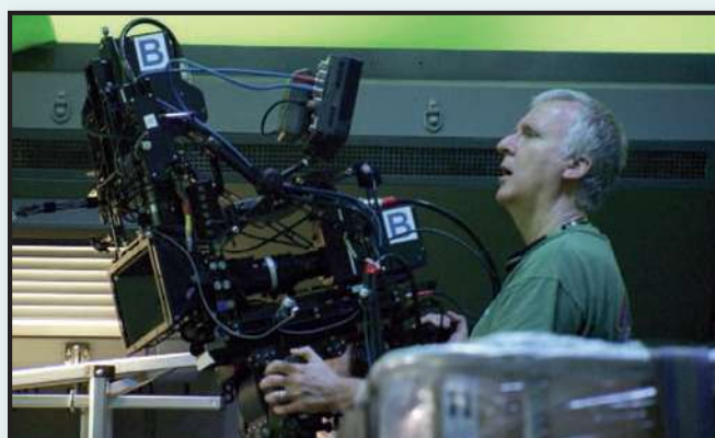
5.66 A 3D camera rig. James Cameron looks into a video viewfinder as he operates the camera system he helped invent for Avatar .
