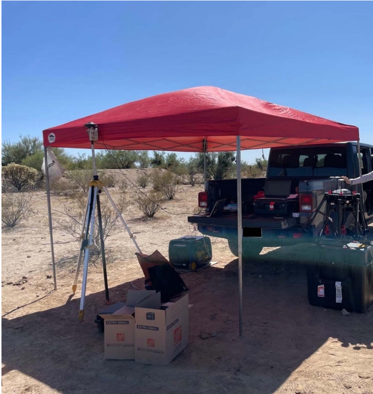
Figure 2. A UAS home-base setup demonstrating the proximity of the transport vehicle, sun cover, and access to a robust generator. Photograph courtesy of Tamas Polanyi.
