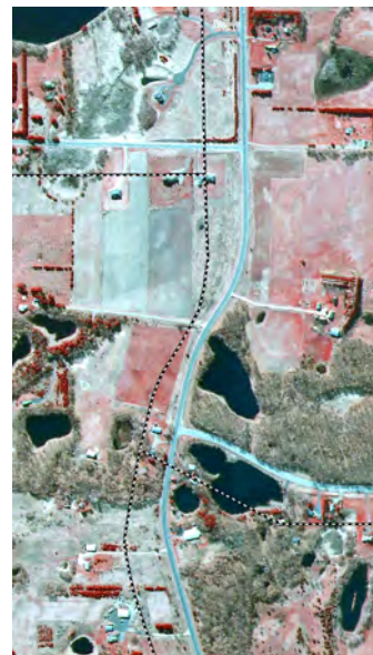
Figure 4-27: An illustration that RMSE should not be used to compare different order transformations, nor should it be used as the sole criterion for selecting the best transformation. Above are portions of a transformed image that was registered to a road network. This area is interstitial to 18 widely distributed control points. Because the 3rd-order polynomial is quite flexible in fitting the points and reducing RMSE, it distorts areas between the control points. This is shown by the poor match between image and vector roads (above right). Although it has a higher RMSE, the first-order transformation on the left is better overall.
