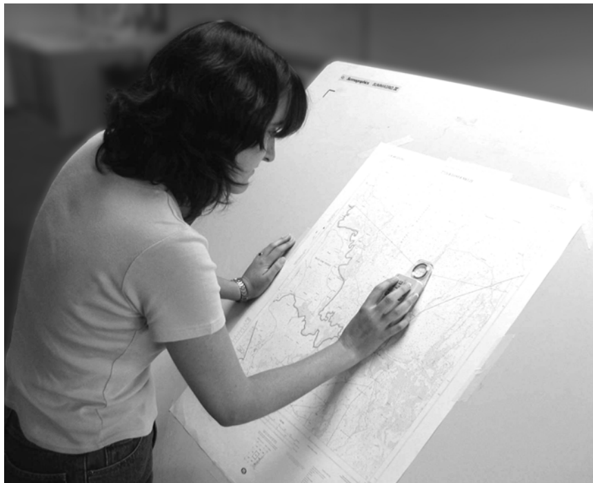
Figure 4-12: Manual digitizing on a digitizing table.
