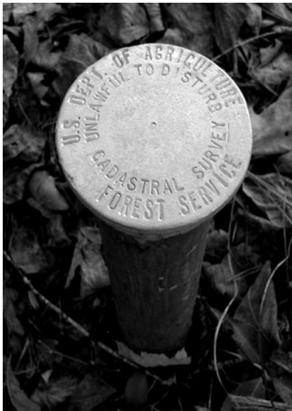
Figure 4-28: Previous surveys are a common source of control points.
