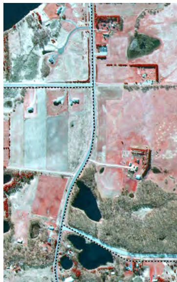
Figure 4-27: An illustration that RMSE should not be used to compare different order transformations, nor should it be used as the sole criterion for selecting the best transformation. Above are portions of a transformed image that was registered to a road network. This area is interstitial to 18 widely distributed control points. Because the 3rd-order polynomial is quite flexible in fitting the points and reducing RMSE, it distorts areas between the control points. This is shown by the poor match between image and vector roads (above right). Although it has a higher RMSE, the first-order transformation on the left is better overall.
