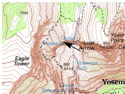
Figure 4-6: Lines on isopleth maps typically do not cross. However, as shown at the arrow in this image, lines may coincide when there is a common value. Here cliffs or overhangs result in converging isopleth lines.
