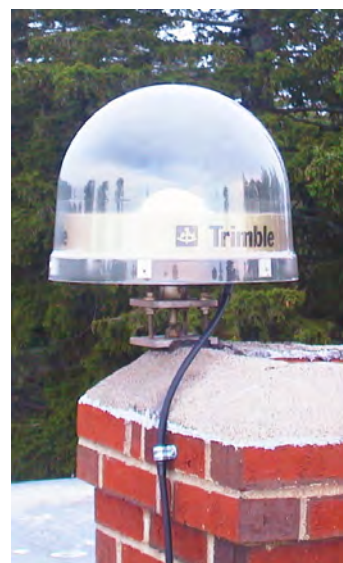
Figure 3-19: A Continuously Operating Reference Station (CORS), used to collect high-accuracy positional measurements from satellites for modern datum development (courtesy NOAA).
