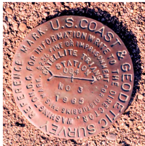
Figure 3-13: A bronze disk used to monument a survey mark.
