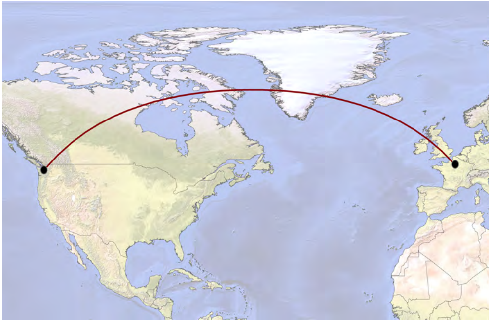
Figure 3-36: Curved representations of straight lines are a manifestation of projection distortion. A great circle path, shown above, is the shortest route when flying from Paris to Seattle, and commonly appears distorted when displayed.
