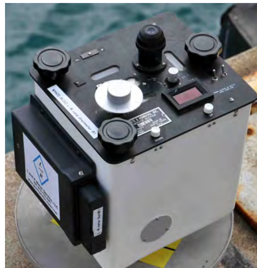
Figure 3-10: A portable field gravimeter, an instrument used for measuring gravitational force at a field location. These measurements are combined with surveying measurements to estimate geoidal surfaces (courtesy National Oceanic and Atmospheric Administration, NOAA).
